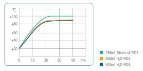
Note: Above data is based on the 220V/50Hz instrument with pure water (H<sub>2</sub>O) and simethicone (Silicon Oil).
